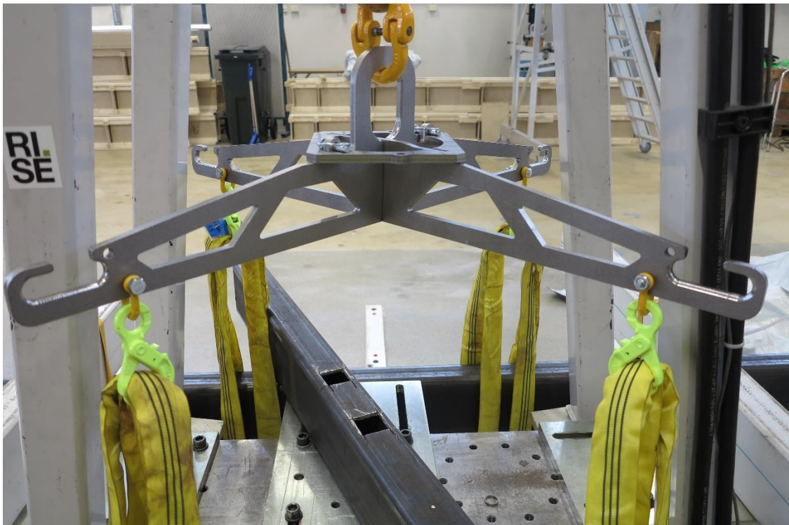
Figure 3. Test set up with lifting hooks.
